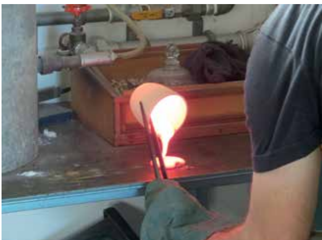
Mark Taylor pouring the experimental glass melts into glass cakes.
