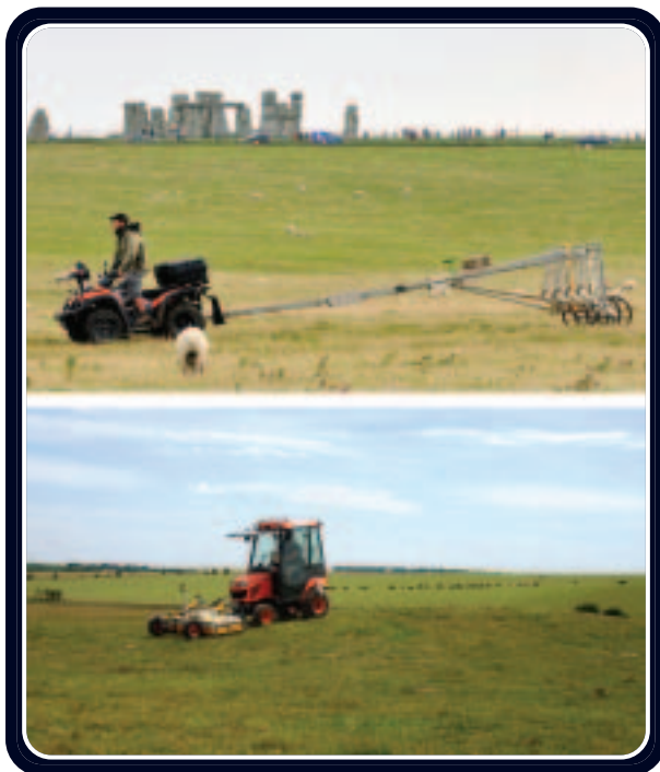
Two of the SHLP motorised geophysical survey systems in operation at Stonehenge: multi-sensor fluxgate-gradiometer array (upper); MALA Imaging ground penetrating radar array (lower).
