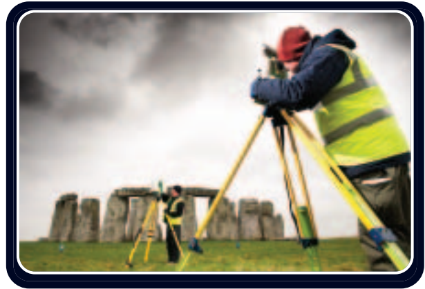
Using the Leica C10 Laser Scanner around the bank and ditch in conjunction with a high-accuracy total station to co-ordinate the scan field targets (photo by James Davies, © English Heritage)
